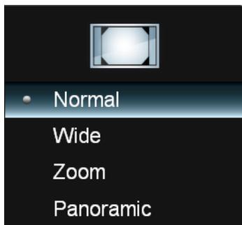
3. Use the ▲/▼ button to select the aspect ratio of the display and press the **OK** button to confirm.
