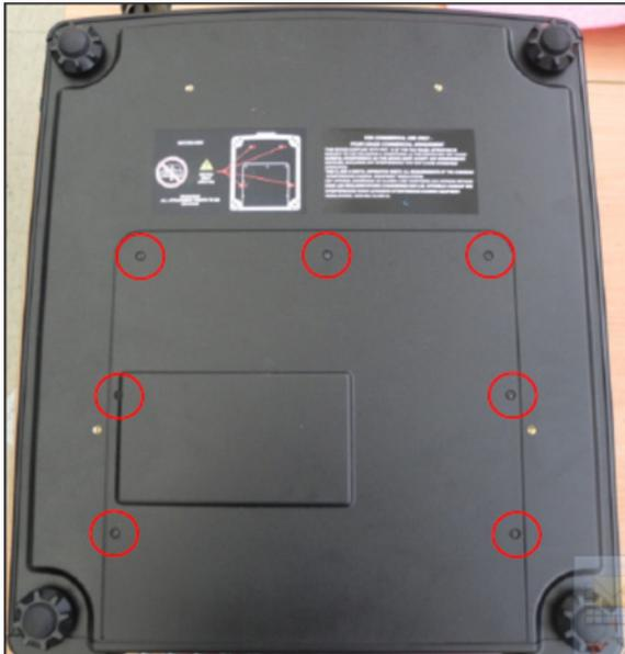
3. Remove and retain the 13 screws securing the main board upper shield. Remove the shield.
