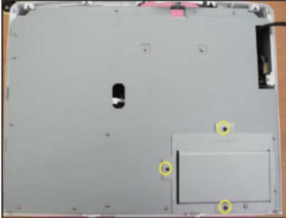
7. Remove and retain 3 screws securing the standard processor (PW610) board. Remove the board.
