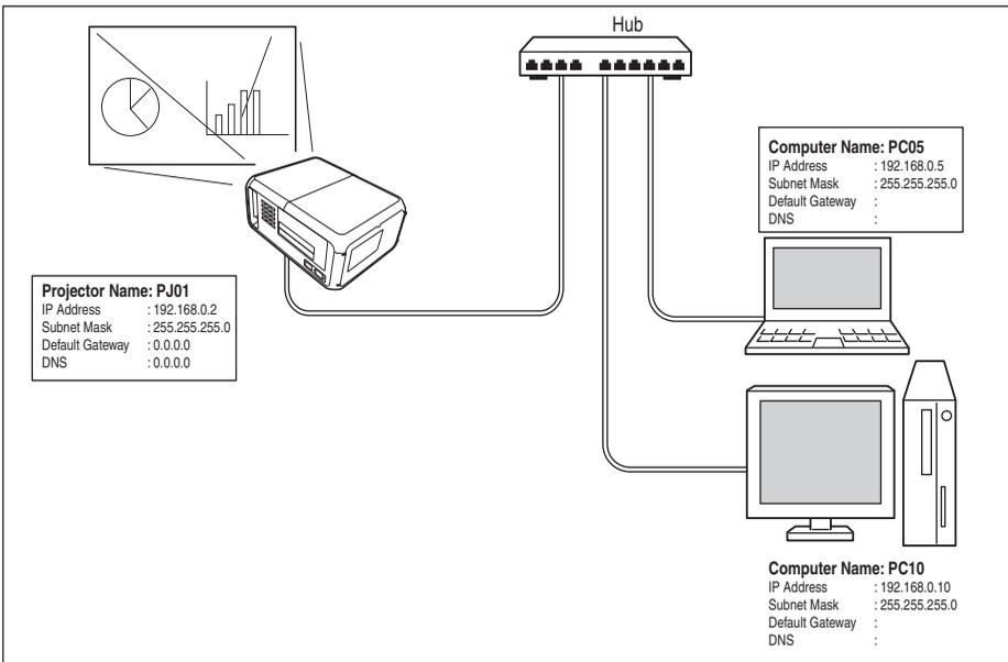
When the projector is connected to the computer directly without hub, the STP crossover cable should be used.
