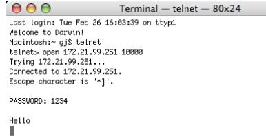
4. Type the commands, refer to below table, to control the projector and then press "Enter" key for termination. For example, type "C00" which is a command to turn on the projector, and press "Enter" key. Confirm the projector is turning on.
