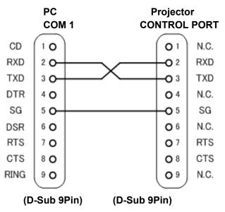
Connect COM port of the computer to CONTROL PORT of the projector. COM Port (COM1 or COM2) of a computer is specified by control software of the computer.
