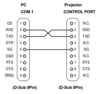
Connect COM port of the computer to CONTROL PORT of the projector.
