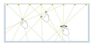
▲ This example of a sensor-based system features sensors along the top (green circles) and infrared LEDs along sides and bottom (blue strips)that allow for precise and accurate detection of touch or object as it enters, hovers within or transitions out of a sensor's field of view.
