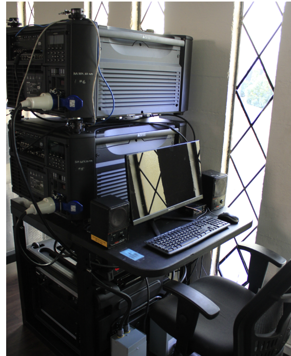
▲ Stacked Christie projectors set up in the Fox Theatre, on a cart custom-made by Tekamaki Photo credit: Tekamaki
