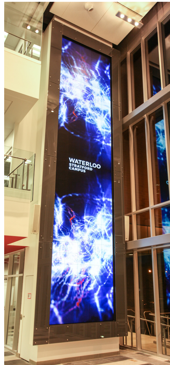
▲ At an impressive 30-feet high by 6.5-feet wide, it's the tallest installation of Christie MicroTiles in the world.
