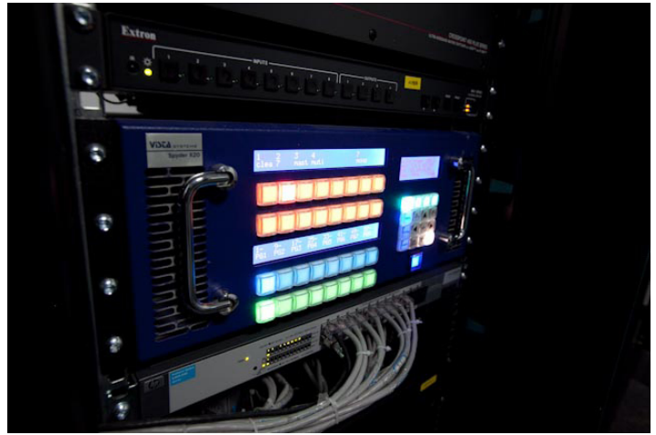
The Christie Spyder X20 was instrumental in the HUST system installation - meeting the requirement for 8-channel stereo sync, defined by the customer.
